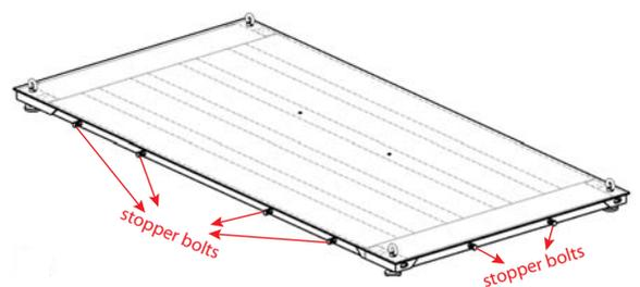
(5) Adjust eight feet height, make sure to keep two platforms on the same level .
