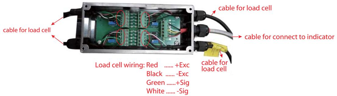
(9) Follow the same step to place the other junction box on the other side of ramp , then joint cables .
