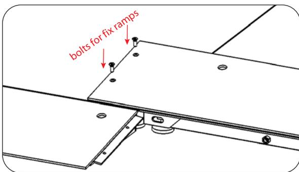
(7) Joint anchor bolts on ramps .
