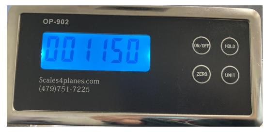
Next press the **UNIT** button. 001950 would appear. Keep pressing the **UNIT** button until 001150 appears.
