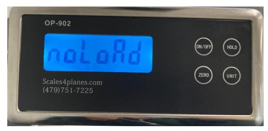
noLoAd will appear. This is the zero calibration. Make sure there is nothing on the scale. Make sure
