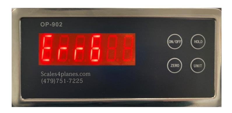
The first step would be to check the wiring.
